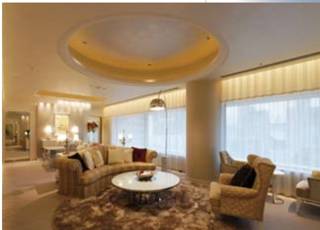
Gradient with 3000K color temperature produces quality light similar to warm incandescent sources.
